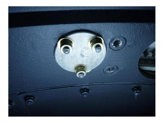
Before continuing, it's a good idea to fit the bolts that will secure the turret to the airframe. Although the AP2799Q says there should be fifteen of these there are actually fourteen and, to complicate matters further, there are sixteen holes in the airframe mount. The extra two holes are actually alignment holes that engage with two special bolts on the turret stops.
