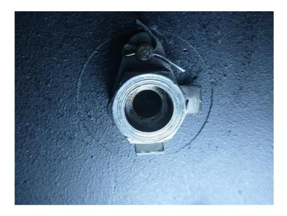
The horizonal rollers are then fitted onto their studs and secured. This removes any lateral movement within the rings.
