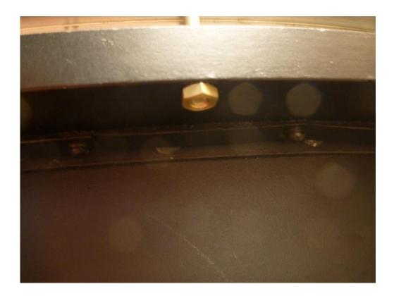
This particular turret has five fittings that also go in at this point, although the AP2799Q only mentions three of them. In general, the rings are held together with countersunk head bolts, with the heads at the bottom – some of these bolts also secure fittings. The fittings include the turret lock and traversing stops (below).
