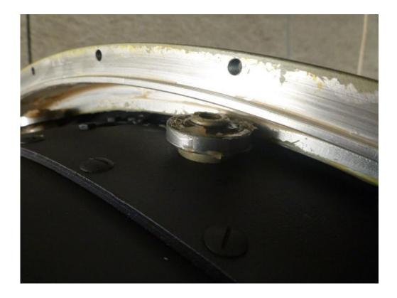
At this point it is essential to fit the special bolts to the rotating ring. These bolts come in three lengths and fit to particular positions depending on how many items they pass through on the accommodation plate. There is absolutely no chance of fitting these later.
