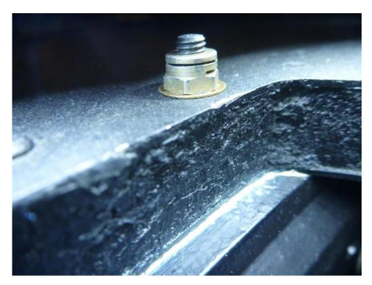
With this done it was possible to try the fit of the turret rings, drum and floor to an original Lancaster reat turret mounting plate. All was in order and assuming the mounting plate fitted to 'Jane is the same there should be no problems fitting the turret.
