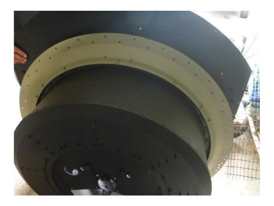
Meanwhile, for a bit of light entertainment, the Dauntless rear gunner's mount was progressed. There was a fair bit of re-manufacturing required here and then the whole thing was sprayed with some left-over primer. The next job for this is to apply the grey finish and bolt the two guns in, after that it just needs to find a display home.
