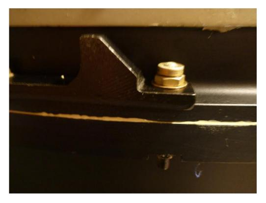
Once bolted up the turret rings, drum and floor assembly could be re-fitted to the stand. It is now possible to fit the accommodation plate to the rotating ring and find out if the three lengths of bolt went into the correct places. Pictured below is the assembly so far with the special bolts protruding and how a correctly positioned bolt should look.
